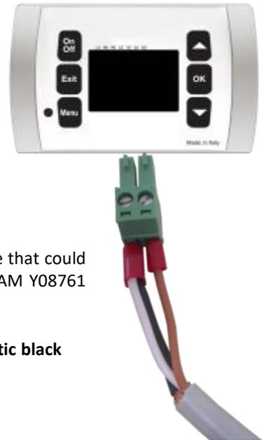
To connect the display, the cable from the unit must be connected as shown on the right:
