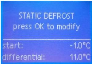
It is used to set the parameters for static defrost operation.
