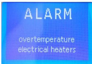
To the left is an example page displaying the alarm, the device in alarm or the type of alarm is shown at the bottom; in this example the electric heating elements are in alarm.
