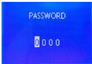
Press at the same time the keys on the right side UP, DOWN and OK. The screen on the left will appear. This screen is prompting for the password. Insert 0099 and press OK to confirm.
