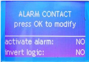
It is used to enable the contact for the alarm and, if necessary, to reverse the operating logic.
