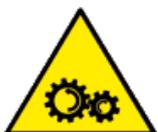
Moving mechanical parts hazard
