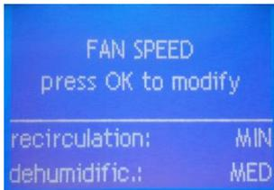
It is used to change the fan speed in the operating phases:
