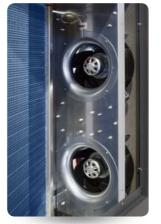
All models of the **NRC** range are factory-fitted with DX coils with hydrophilic treatment of the fins. The particular coating, combined with proper design of the air flow passage velocity, encourages condensate collection during the dehumidification process, thus avoiding water drops being dragged outside of the unit.
