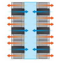
• the "In Row" configuration, where cold air is released in the «cold aisle» towards each rack unit and the hot air is extracted by the rack cooler in the "hot aisle".
