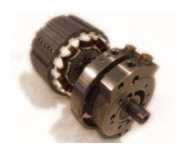
The Brushless synchronous motor has "no brushes" as the power is only sent to the stator and not directly to the rotor, therefore, sliding electrical contacts are not required. Over 20 Hz, the mP on board controls a feedback signal (BEFM Back Electro Motrice Force) that can certify the rotor's synchronous rotation with a magnetic field and implements anv torque corrections to restore/maintain synchronism and therefore maximum efficiency.
