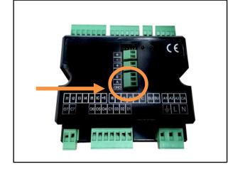
Use a CEAM Y08761 cable or equivalent to connect the entire Modbus network.
