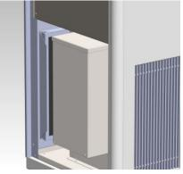
Tilt the filter and pull it out. Also incline the sequence for the right filter
